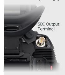
The 3G-SDI output terminal (BNC connector, 5CFV) can be used to transmit FHD 1080/60p, 1080/50p signals through a coaxial cable over a distance of up to 100 m. Panasonic recorders equipped with SDI input can be linked to the Rec Start/Stop function of the AG-CX10/HC-X2000.
